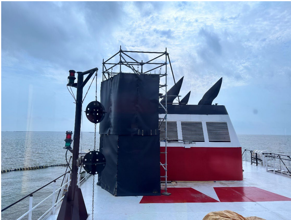
Photograph 1. Hydraulic Dredge Sound Mitigating Measures
