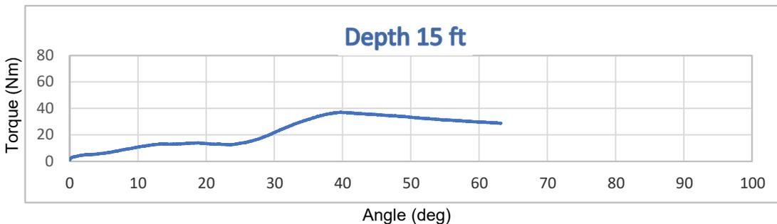
Shear strength = 23.80 [kPa], Max torque = 37.13 [Nm], Rod friction = 13.16 [Nm]
